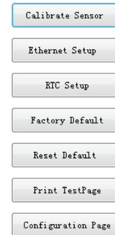
4. Select the media type (Gap/Black mark / Continue) and calibration type (Auto/Manual) to calibrate the sensor specified in the printer setup group media sensor field. For the general media you only need to select the media type then click the “Calibrate” button.
