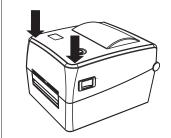
(4)Feed the paper printing side face up, the label leading edge onto the platen roller. Move the media guides to fit the label width.
