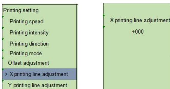
Use this option to adjust the printing position and the stop position of the label.
