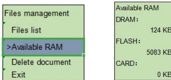
This option can be used to check the residual memory space.
