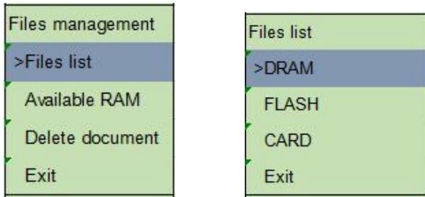
This option can be used to display, delete, and execute (.BAS) the files stored in the memory.
