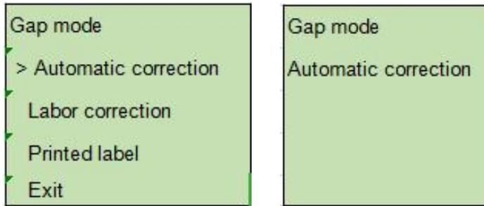
When entering this option, the above message will appear, and the printer will feed 2-3 sheets of label paper for calibration of the sensor. When the calibration is completed, it will return to the previous menu.
