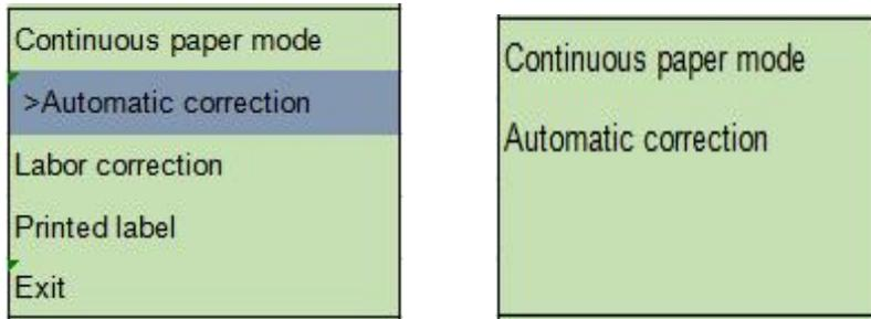
When entering this option, the above message will be viewed, and the printer will automatically calibrate the sensor for the paper. When the calibration is completed, it will return to the previous menu.
