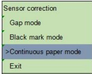
Press SCROLL UP and SCROLL DOWN to select the type of sensor, and press MENU to complete the setting.
