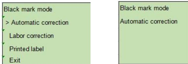
When entering this option, the above message will be displayed on LCD display screen, and the printer will feed 2-3 sheets of paper for calibration of the sensor.
