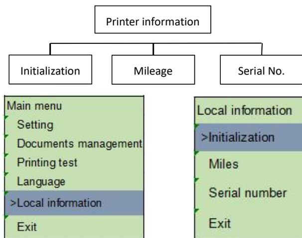
This option can be used to initialize the printer or check the serial number and the mileage printed.
